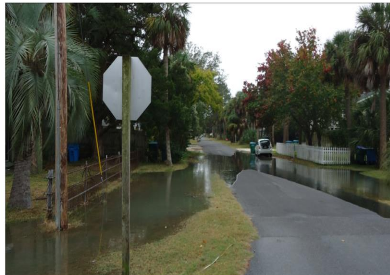
FIGURE 4.7: SALTWATER FLOODING OF YARDS AND STREETS FROM STORMWATER DRAIN DISCHARGE DURING KING TIDE, NOVEMBER 14, 2012
